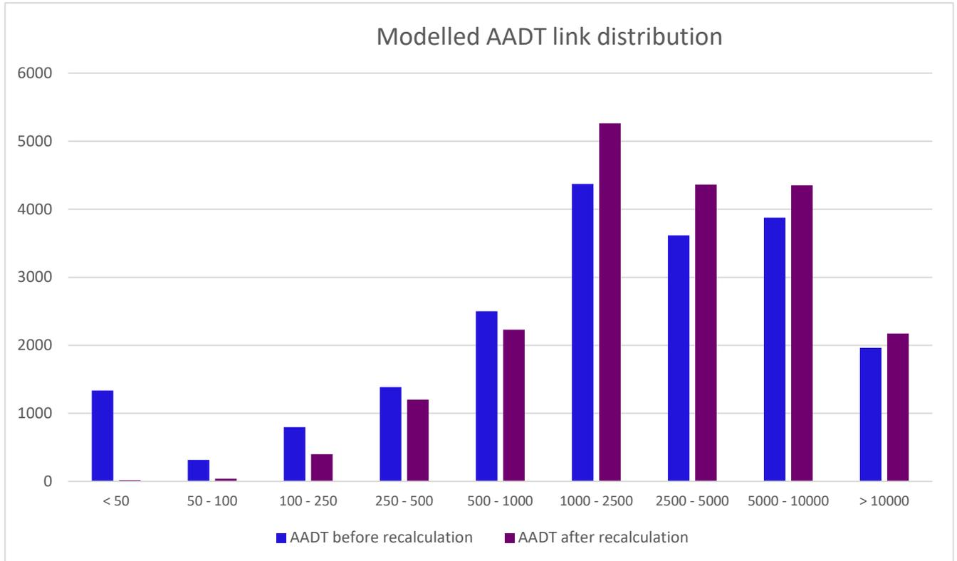
Diagram 5.11 Link distribution Diagram before/after on AADT difference
