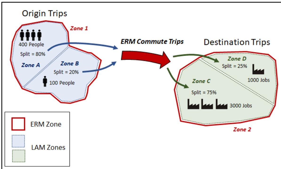
**Diagram 6.5 LAM Disaggregation Example – AM Peak Commute Trips**
