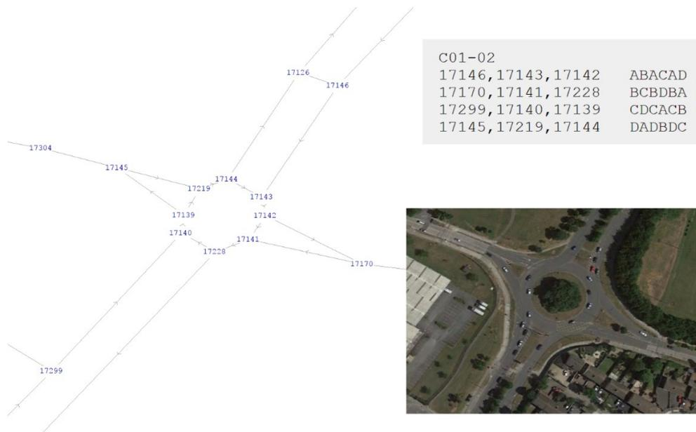
**Diagram 5.3 Bus Connects LAM Node Matching (Junction C01-02)**
