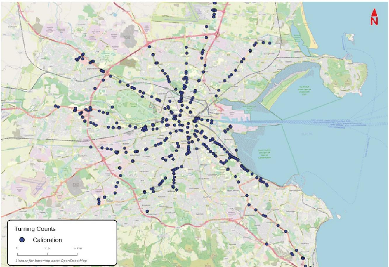
**Apx Diagram A.1 Turning counts used in Calibration**
